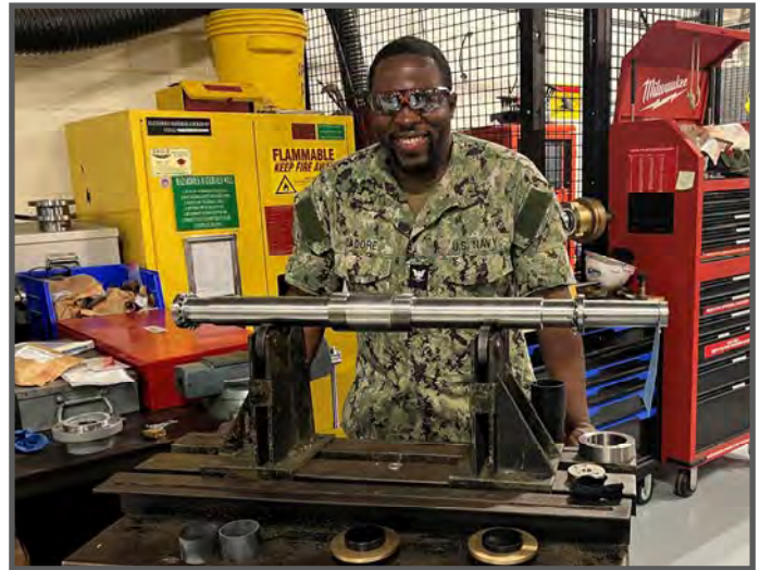
Mid-Atlantic Regional Maintenance Center's (MARMC) Machinery Repairman Third Class Colson Cadore smiles for a photo featuring the pump shaft he recently machined from a piece of square Monel bar. (Photo courtesy of MARMC Commanding Officer, Capt. Jay Young.)
