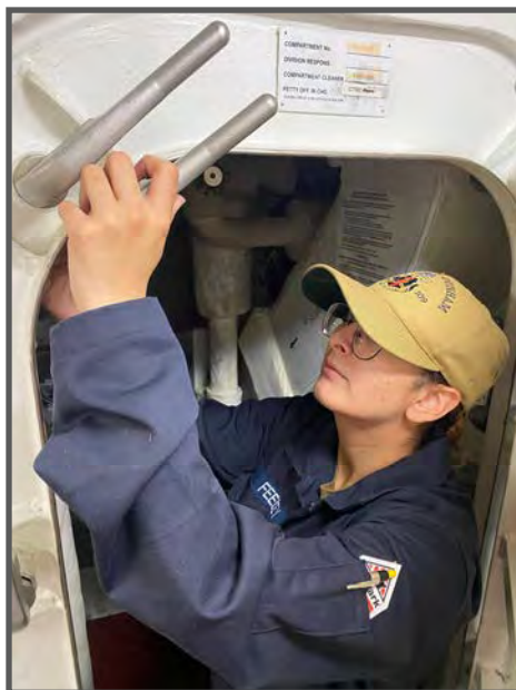
USS Jason Dunham's (DDG 109) DCFN Aaliyah Feeley checks an individually dogged watertight door bushing for proper alignment. (Photo by Rick Smith, Afloat NAMTS Inside Machine SME.)
