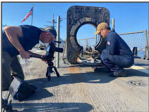
BM2 Alpha Yee inspects and lubricates a flush and ramped low profile (RLP) steel watertight hatch and scuttle (quick-acting) and prepares to perform a test procedure. His step-by-step actions per a maintenance requirement card (MRC) were recorded by videographer, Paul Del Signore, for the development and production of job performance aids (JPA) to be used by U.S. Navy Sailors. (Photo by Darius Mitchell.)
