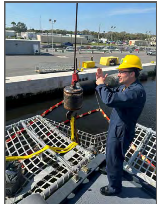
SERMC's BM2 (SW) Brice Smith is aboard USS Marquette (LCS 25) as he sends a signal to the crane operator weight testing flight deck nets. (Photo by BM2 (SW) Jazzment Shanks.)
