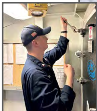
MM3 Matthew Davis adjusting CCS QAWTD 2-42-2 using Method 2. (Photo by Ramir Pulido.)
