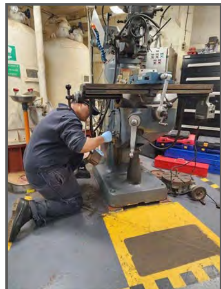
MR3 Robert Figueroa is preparing to install a lubricator holding unit for the Bridgeboard Milling Machine after conducting an after lubricating filter inspection aboard USS Harpers Ferry (LSD 49).
