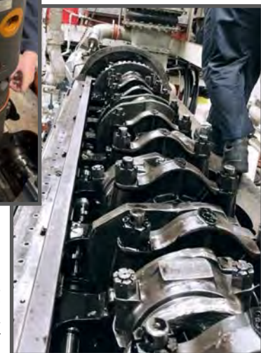
The Fairbanks Morse opposing piston diesel engine utilizes a massive crankshaft that is precision honed to be both strong and balanced. (Photo by EN1 (SW) Kevin Mellor.)
