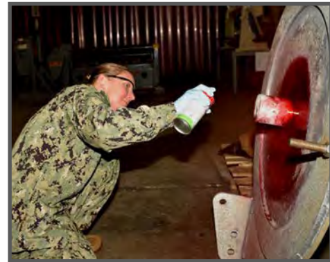
Above: Hull Technician 1st Class Petty Officer Jennifer Schleuning sprays penetrant on an upper platform for a ship's brow while conducting non-destructive testing at Southeast Regional Maintenance Center (SERMC) in Mayport, Fla.
