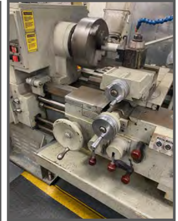
After 6 years, the Clausing AVS 2013 lathe aboard USS Stout, is fully refurbished and has been returned to operating condition by the combined self-sufficiency efforts of Ship's Force, NAMTS/NATA Subject Matter Experts, and technical assistance of Defense Logistics Agency's Industrial Plane Equipment program in Mechanicsburg, Pa.
