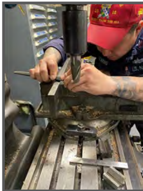
MR1 (SW) Thomas Evans sharpens a blade for the HT's Iron Worker. (Photo by Rick Smith.)
