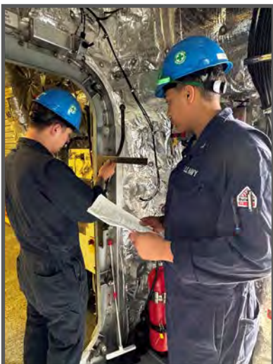
DC3 Devin Rivers (right) and DCFN Noah Steadman conduct a knife edge inspection on a Quick acting Watertight Door on board an Independence variant LCS.
