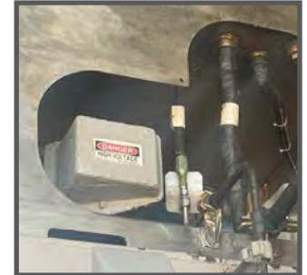
Left: Severe corrosion on an electrical junction box on the main deck affecting the ship's lifesaving system. Note that the bottom of the box cover had heavy corrosion, which could have been affecting the structural integrity of the high voltage box. Right: The same electrical junction box after it was cleaned then treated with Sailor Putty and Sailor Paste; this is a temporary remedy to prevent further corrosion until the unit can be repaired or replaced.
