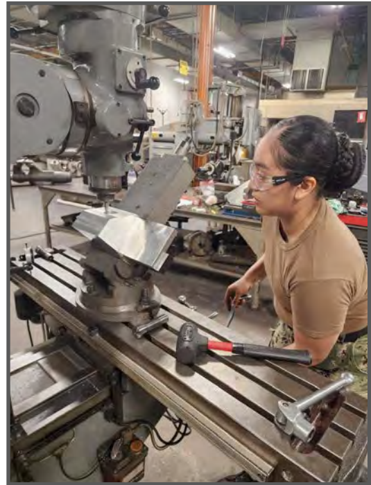
MR2(SW/AW) Mayra Zepedaalvarez uses a Bridgeport Vertical Milling Machine to cut a shape aluminum stock to design specifications. Once completed, this part will be sent to USS Washington (SSN 787) for installation. (Photo by MR1(SW) Taylor Bowie.)
