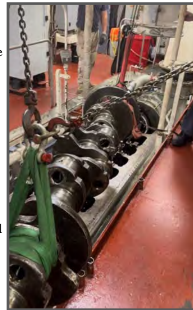
The diesel crankshaft is extremely heavy and needs to be lifted up and away from the engine as carefully as possible. Engine spaces can be cramped but with well-practice rigging techniques, MARMC Sailors were up for the task. (Photo by EN1 (SW) Kevin Mellor.)
