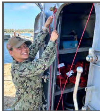
An Expeditionary Strike Group 3 Sailor from Assault Craft Unit 1, Damage Controlman 1st Class Dana Briski, who is enrolled in the NAMTS Watertight Closure Maintenance Technician JQR, conducted a twist inspection using NSTM 600 Volume One's Section 600-2.5 Knife Edge Inspection using the String Method (left) and conducted a knife edge height inspection of a quick acting watertight door IAW MRC 1671/008 Q-5 (right) in March. (Photos by Ramir Pulido.)
