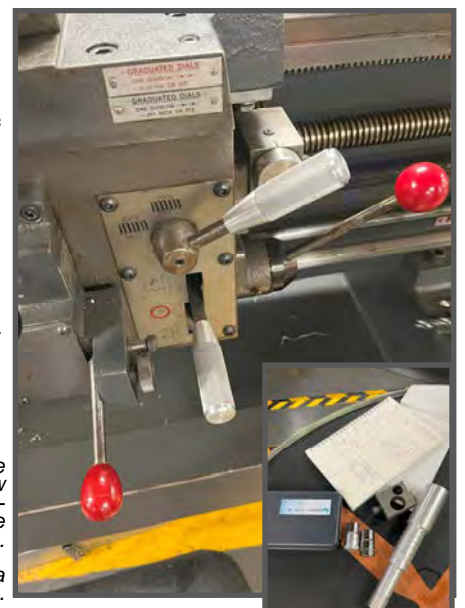
A look at one of the lathes sporting new handles that were manufactured as part of the knurling challenge.
