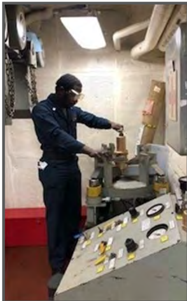
MM2 Armstrong Calixte from Port Au Prince, Haiti adjusts the pressure on relief valve for Nr.1 Expansion tank for forward air conditioning plant while conducting a pop test using the ship's valve test stand.
