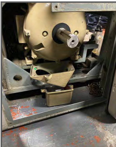
A new electrical motor is installed in a Clausing AVS 2013 lathe aboard USS Stout, by EMC(SW) Emmanuel Zuniga along with MRFN Bryan Rivera.
