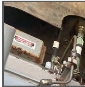
Left: Severe corrosion on an electrical junction box on the main deck affecting the ship's lifesaving system. Note that the bottom of the box cover had heavy corrosion, which could have been affecting the structural integrity of the high voltage box. Right: The same electrical junction box after it was cleaned then treated with Sailor Putty and Sailor Paste; this is a temporary remedy to prevent further corrosion until the unit can be repaired or replaced.
