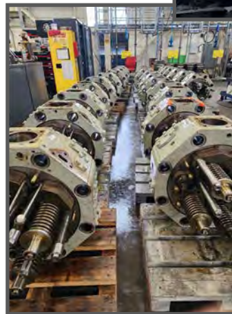
Cylinder heads coated with CPC 500.
