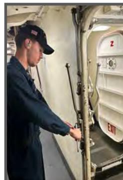
Left: USS Ashland's SWCN Sean Jones II adjusting a Watertight Door Operating Lever IAW NSTM 600 Volume One Section 600-2.2.3.5.2 and MRC1671/0 08 S-12 and U-6. (Photo by Ramir Pulido.)
