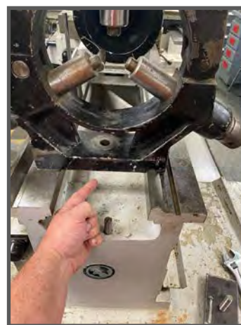
Left: NAMTS Inside Machinist mentor points out to HTFN Malkowski that the Lathe steady rest mounting bracket was missing.
