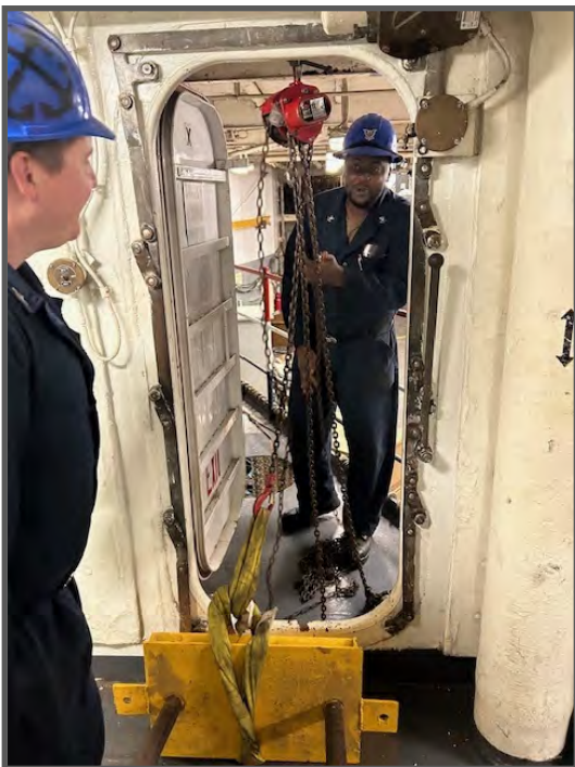
BM1 Kindrick and BM2 Oneil conduct the 300 series Rigger Weight Tester NEC through ships rigging as part of their efforts to earn their NEC. (Photo by Brian Epling.)
