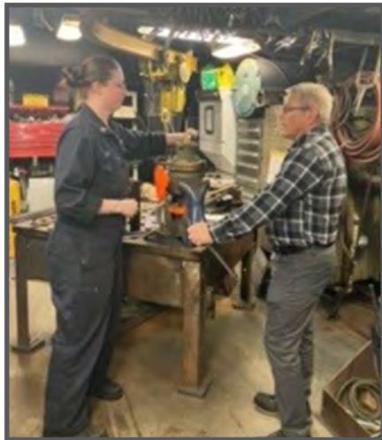
HT3 Kali Riley from Blue Ridge, Texas, removes the adjusting screw for ballasting system relief valve BALR-V-002 as NAMTS Afloat Outside Machine SME Mike Dengate provides guidance on the disassembling process for a relief valve. (Photo by Steve Constantino.)
