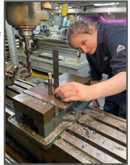
HTFN Malkowski manufacturing Lathe steady rest mounting bracket. (Photo by Rick Smith.)
