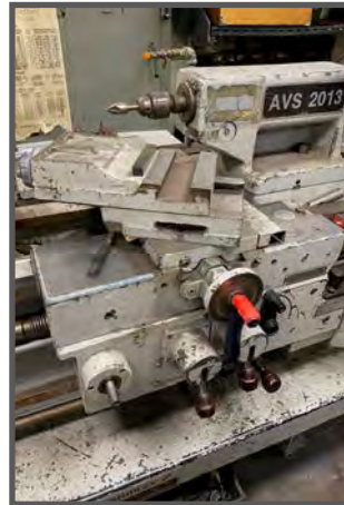
A Clausing AVS 2013 Lathe, aboard USS Stout (DDG 55), missing handles for the saddle and compound rest assemblies, in addition to a missing Tool Post holder.
