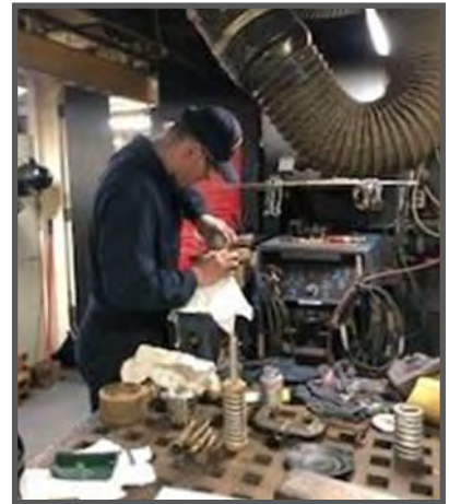
HTFN Daniel Chmielecki from Connecticut removes the bluing compound from the seat of relief valve FL-V-2-102-13 after conducting a contact check of the seat and disk.
