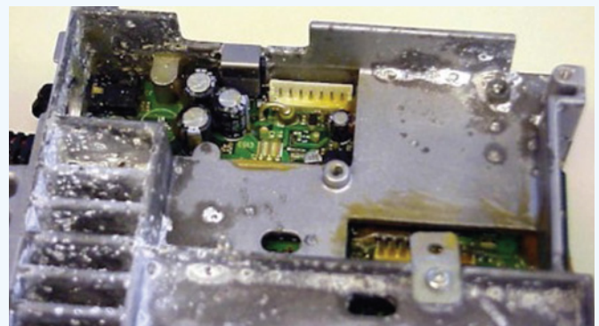
Unprotected Circuit, Heavily Corroded
