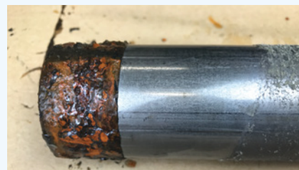
After 1000 hrs of ASTM B117-18 Salt Spray Test
